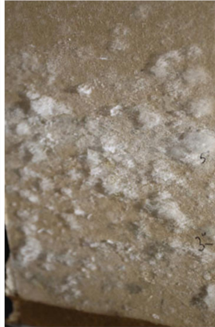
Back side of same piece of drywall. Lots of mold after 7 days.
