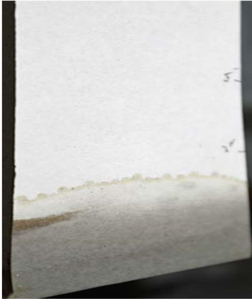
Front of Drywall inserted into 1" of water for 5 days. No mold.
