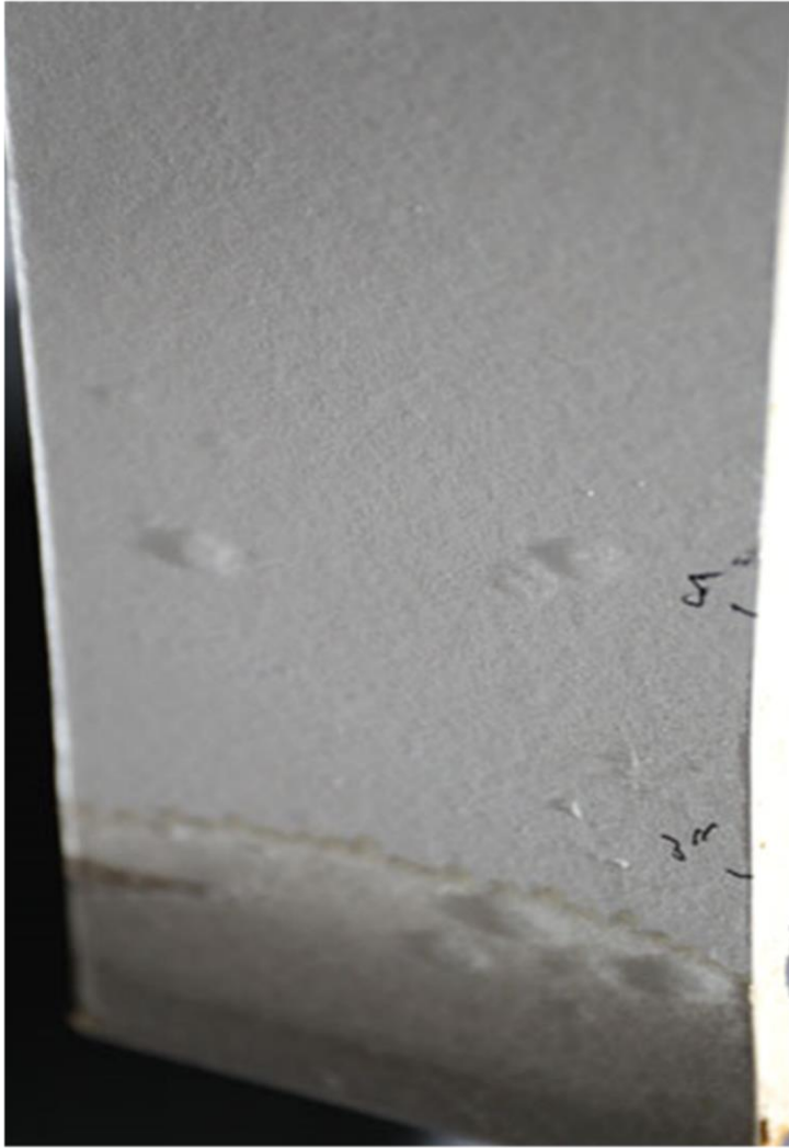
Front side of Drywall inserted into 1" of water for 7 days. No mold.
