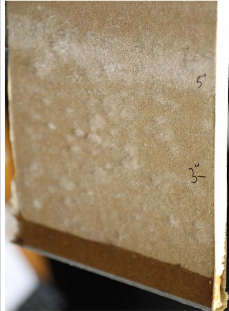
Back of same piece of drywall. Mold after 5 days.
