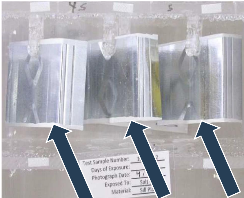
Photo 5: Sill plate in salt water Day 0
