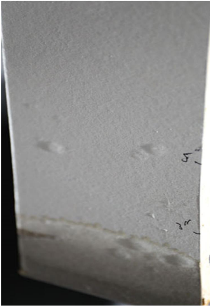
Front side of Drywall inserted into 1" of water for 7 days. No mold.
